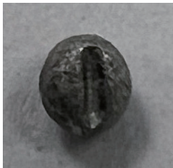
图16 混合悬浮熔炼后的样品形状 Fig. 16 Sample shape after mixed levitation melting
